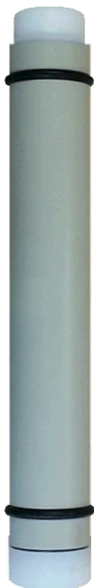
Acoustic logger (600 x 95mm)
