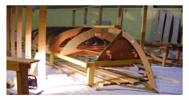
THE BUILD FRAME AND MOULDS
